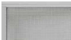
PERFORATED ALUMINUM† 0.312" square perforations on ½" centers
